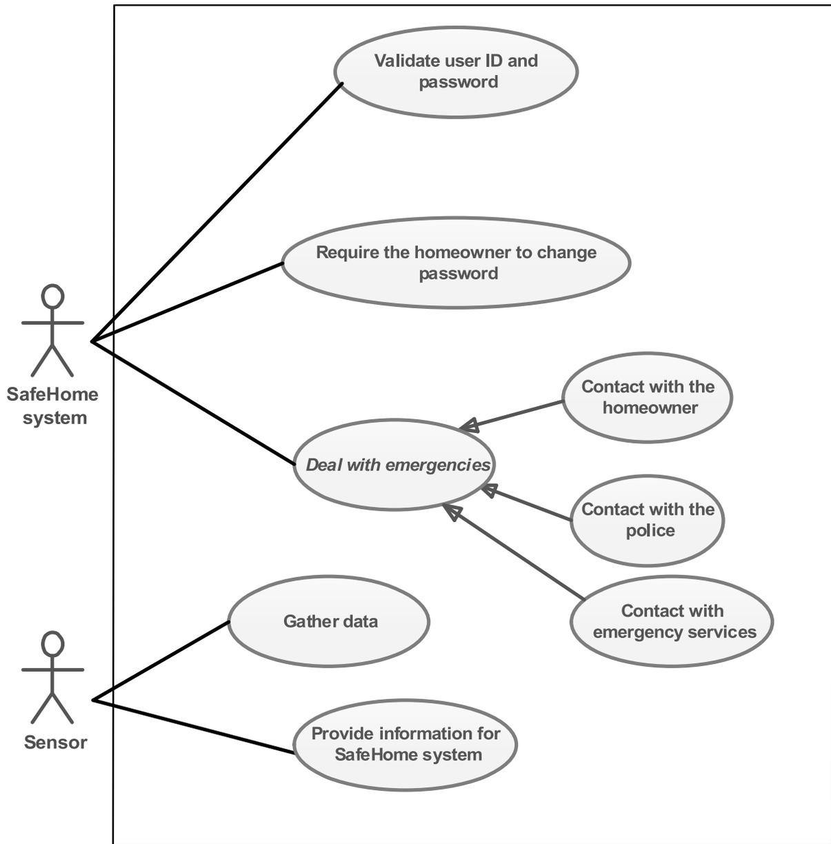
**Figure 2: Use-case diagram for Security feature (SafeHome system and sensor are actors)**
