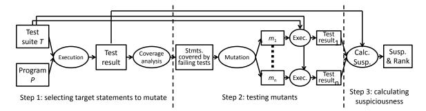
Figure 4.2: Framework of MUtation-baSEd fault localization technique (MUSE)
