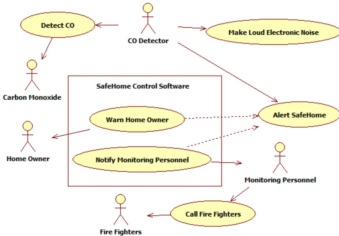
Figure D-4 – Use Case Diagram for Monitoring Carbon Monoxide (CO)
