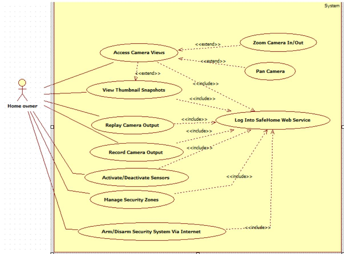
Figure D-7 – Use Case Diagram for SafeHome Web Service
