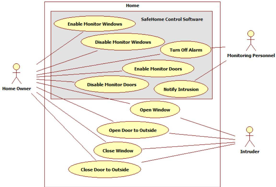
Figure D-1 – Use Case Diagram for Monitoring Windows and Doors
