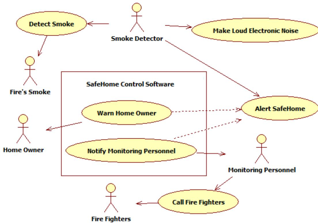
Figure D-3 – Use Case Diagram for Monitoring Fire and Smoke
