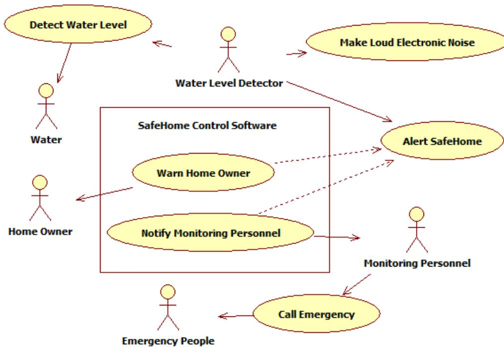
Figure D-5 – Use Case Diagram for Monitoring Water Levels
