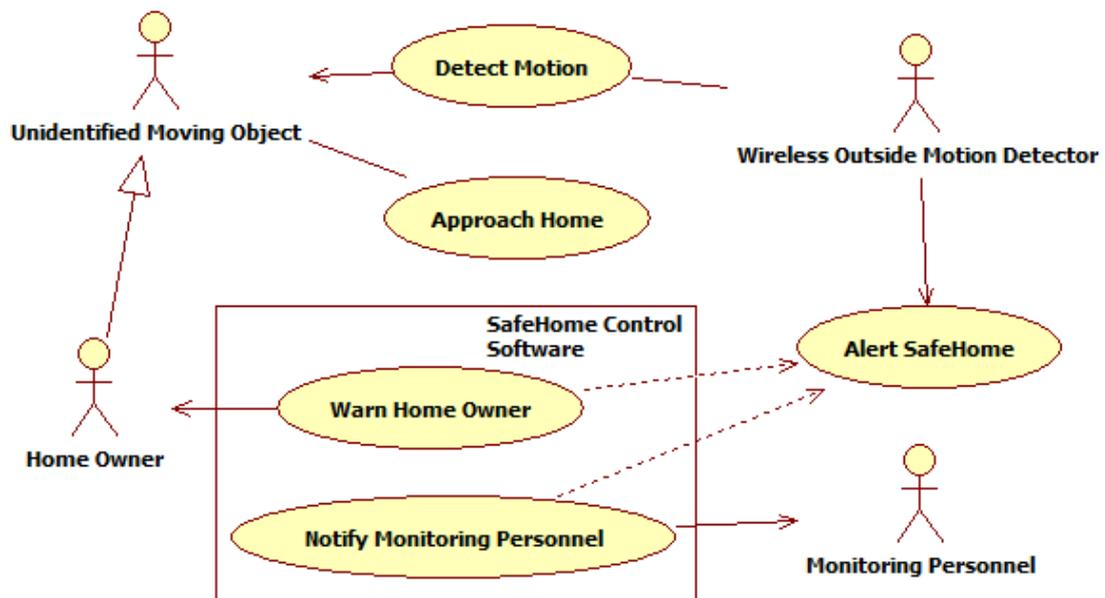
Figure D-2 – Use Case Diagram for Monitoring Outside Movement
