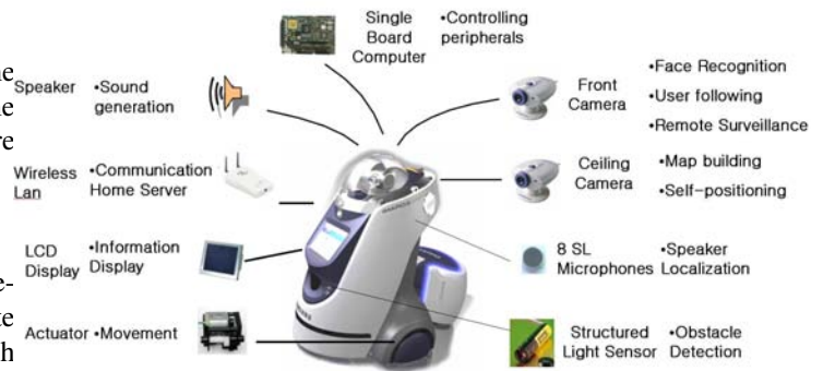
Fig. 1. Components of SHR100
